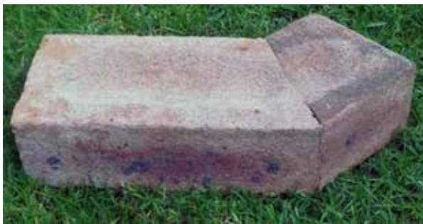
A Cut and Bonded External Angle
